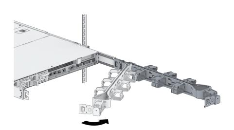
Press on the indicated spot on the outer fastener to unlock it, then slide it away from the connector base.
