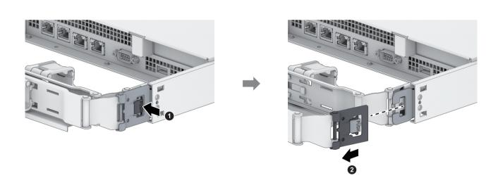
Press on the indicated spot on the inner fastener to unlock it, then slide it away from the connector base.
